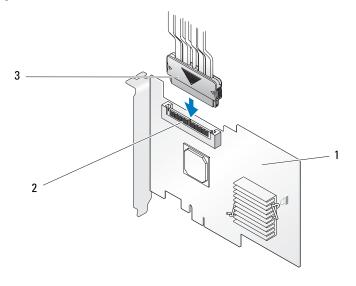
1 SAS 5/iR Adapter 2 SAS x4 internal connector 3 cable
